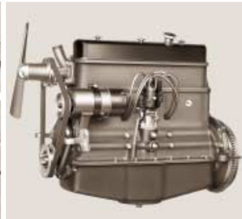
Foundation of success: the 1.2-litre six-cylinder engine with 30 bhp.
