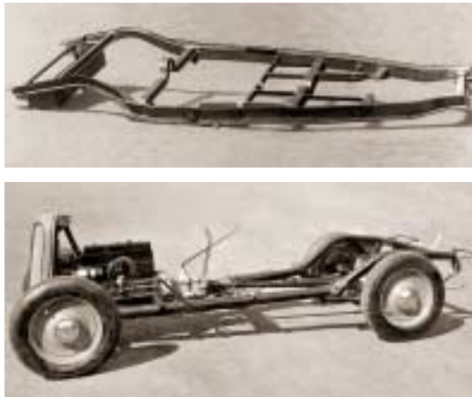
Top: the first test chassis frame for the BMW 303. Bottom: the new lightweight tubular frame design for the series.
